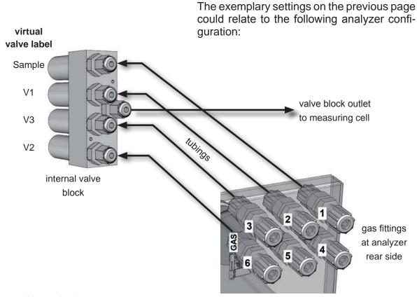
Fig. 7-3: Internal Valves Assignments
